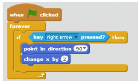
Figure 51: Code to start Cat1 moving to the right of the track
